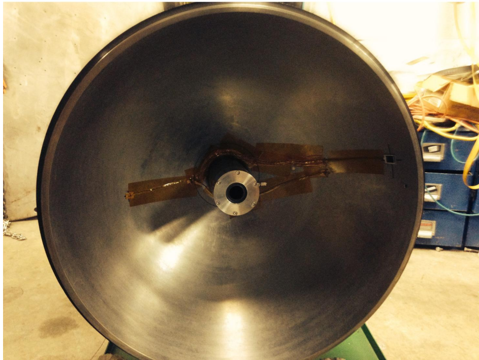
Figure 1.2: Interior of the 60cm Setup taken apart showing electronics mounted inside, before assembly. The setup tries to minimize the invasiveness of the electronics. The axis of rotation, embodied by the physical axle, is vertical during operation. Photographs courtesy of Matthew Adams.
