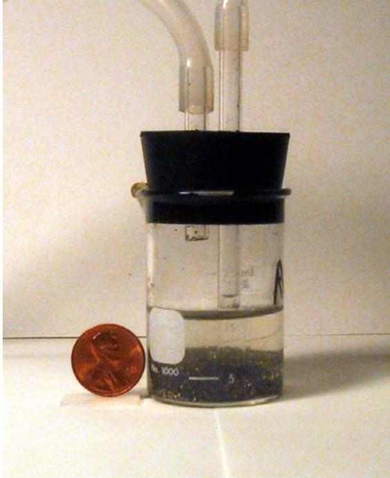
Figure 4. Bacteria reaction vessel. 5.0 grams of pyrite are in the bottom. A glass tube was suspended above the liquid line to bring fresh input solution into the vessel. Another glass tube was suspended just below the air/ water interface to remove output solution. Cotton was not used because it would have introduced organics into the system that might have interfered with bacterial growth.
