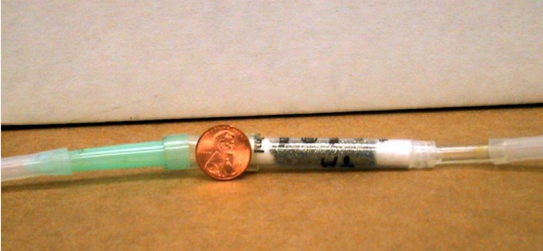
Figure 2 A close-up view of a pyrite column reaction vessel. The length of the vessel is 2.25 inches. Each end is packed with sterile cotton to prevent the pyrite from escaping the vessel. The vessel is a modified, sterile syringe. Various sizes of tubing and a pipette tips were used to modify the system and create a continuous flow.
