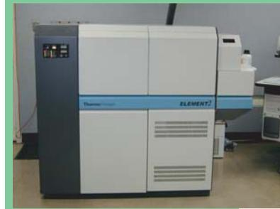
Inductively Coupled Plasma - Mass Spectrometer with a single electron multiplier detector
