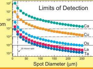
Element detection limits are a function of spot size, mass of the isotope, and the element's 1<sup>st</sup> ionization potential (ip). Ca, La, and Ta have similar 1<sup>st</sup> ip, while Os and Ta have similar masses.
