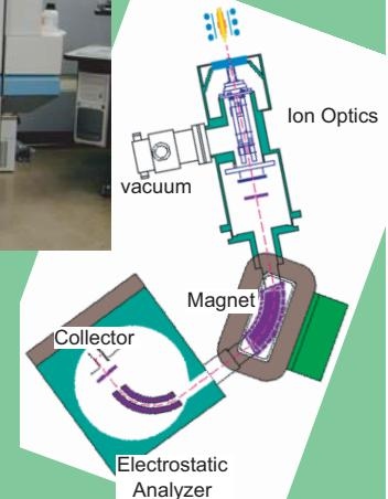
Inductively Coupled Plasma - Mass Spectrometer with a single electron multiplier detector
