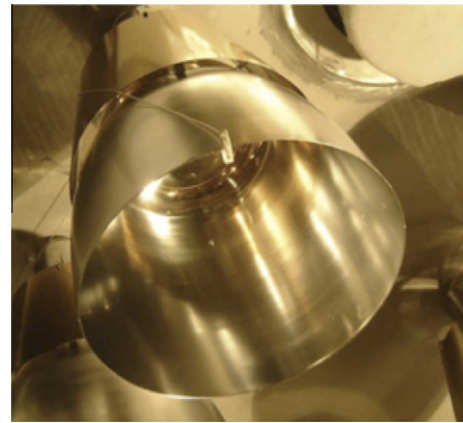
Fig. 8. Winston cone type light concentrator used in Borexino, increasing the effective photon collection area by a factor of 2.5 (courtesy of Borexino).
