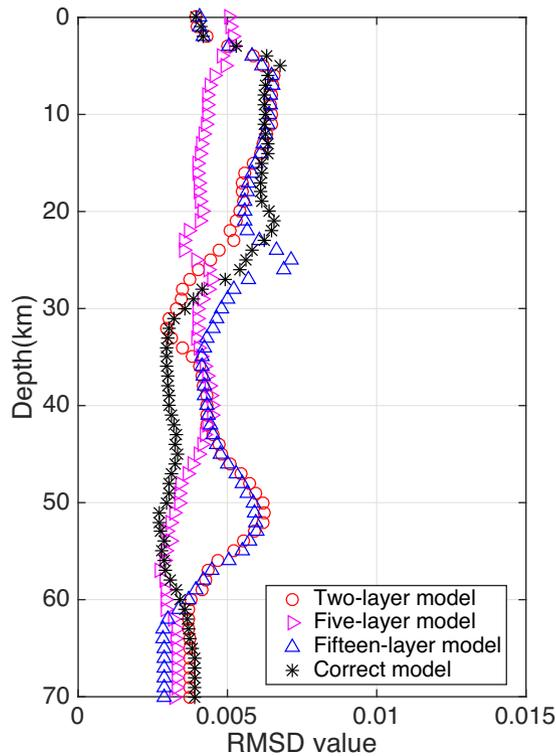
**Figure B2.** Root-mean-square deviation of  $V_s$  posterior probability density functions from TB inversion of surface wave dispersion using four different starting models. We use the following equation to calculate to root-mean-square deviation (rmsd) for the four ensembles.
