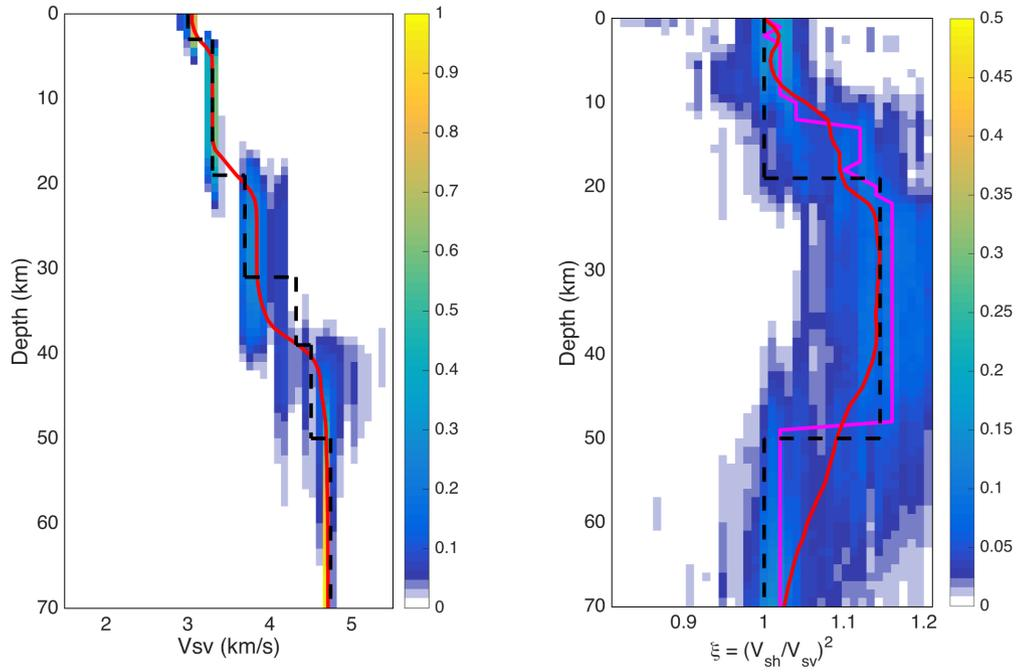
**Figure 12.** Anisotropy inversion with independent parametrization and no scaling on  $Vp$ . The ensemble solutions ( $Vs$  on the left and  $\xi$  on the right) are displayed as probability density functions at each depth, with warmer colours corresponding to higher posterior probabilities, the solid red line denoting the 5 per cent trimmed mean of the posterior and the magenta line denoting its mode. The target model (black dashed lines) is used to generate synthetic data.
