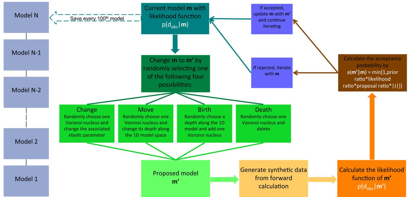
**Figure 2.** A schematic overview of the reversible-jump Markov Chain Monte Carlo algorithm used for inversion. Every 100th model is saved to the ensemble solution to increase the independence of sampled models.
