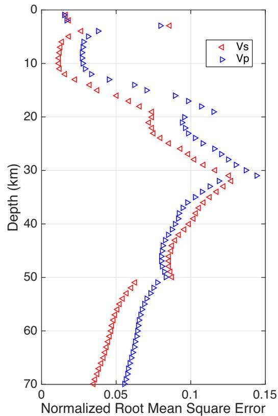
**Figure C1.** Normalized root-mean-square error of  $V_s$  (red) and  $V_p$  (blue) inversion ensemble against the input model. The ensemble is taken from test shown in Fig. 5 where  $V_s$ ,  $V_p$  and density are inverted using SWD and ZH ratio. The rmse of  $V_s$  and  $V_p$  are normalized by their mean at that given depth.
