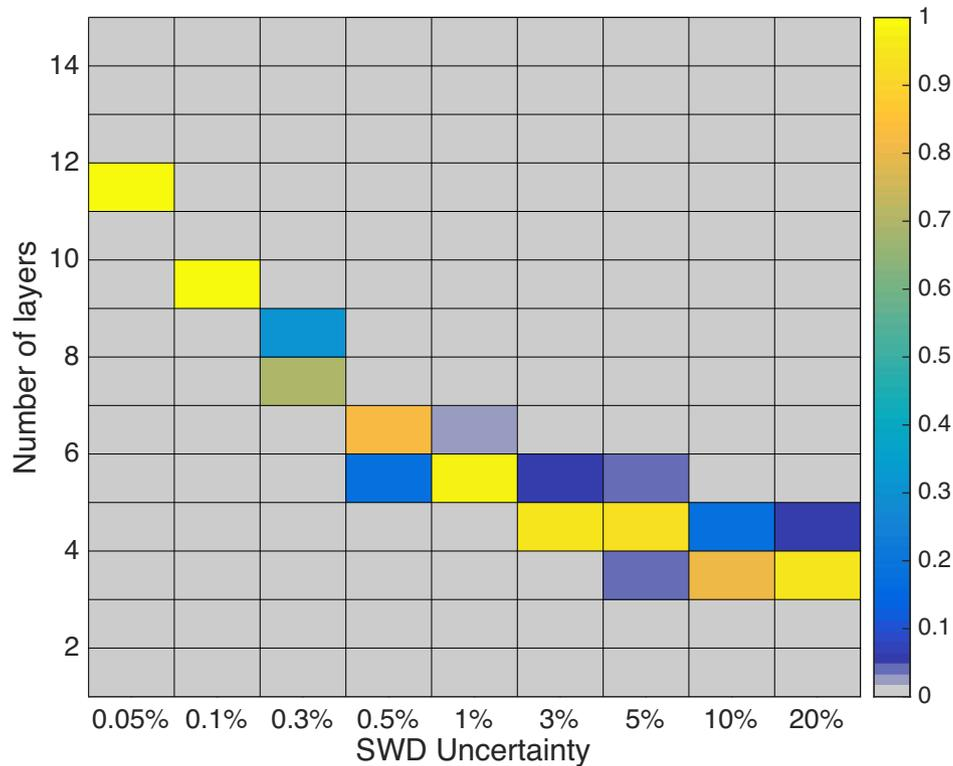
**Figure 9.** Posterior probability distribution of the number of layers in the retrieved ensemble for transdimensional inversion of surface wave dispersion measurements with different measurement uncertainties. The period range of both Rayleigh and Love wave dispersion used is 2–100 s.
