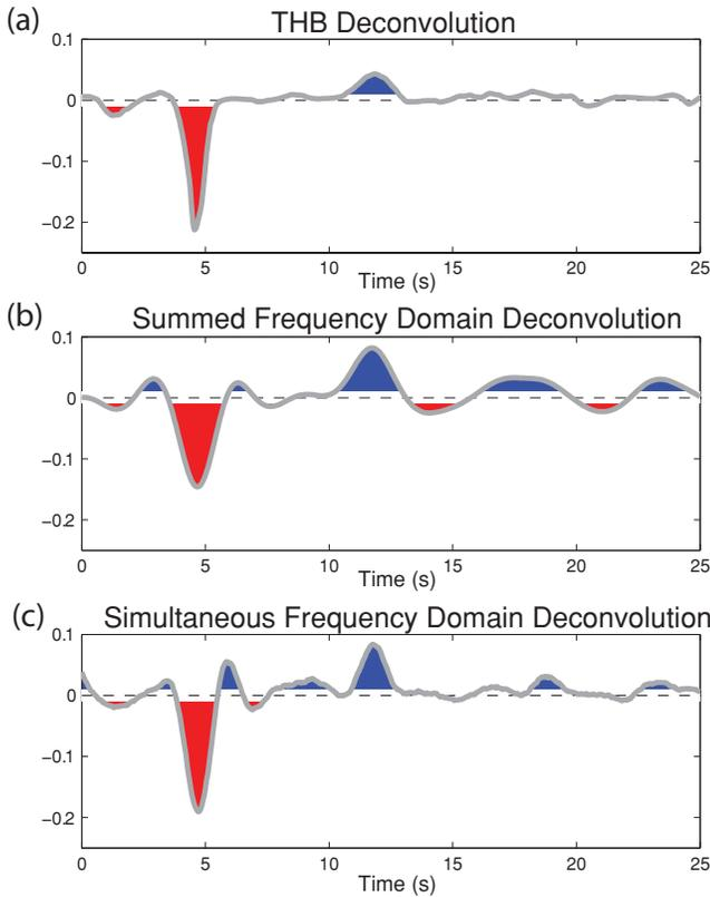
**Figure 11.**  $S_p$  receiver functions from 20 waveform pairs contaminated with high levels of noise. (a) Average receiver function generated using our THBD algorithm. (b) Receiver function generated by averaging individual frequency-domain receiver functions in the time domain. (c) Receiver function generated by simultaneous deconvolution of the waveforms in the frequency domain. Note the absence of artefacts in the THBD result, which yields more easily interpretable receiver functions.
