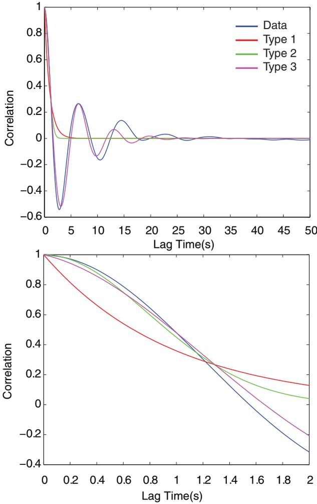
**Figure 5.** Noise correlation from actual noise versus parametrizations as a function of lag time. Parametrization 3 (with  $\lambda = 0.2$  and  $\omega_0 = 4.4$ ) fits the real noise correlation best for all but the smallest lag times, where parametrization 2 fits the real noise correlation slightly better. Parametrization 1 yields poor fits at all lag times.
