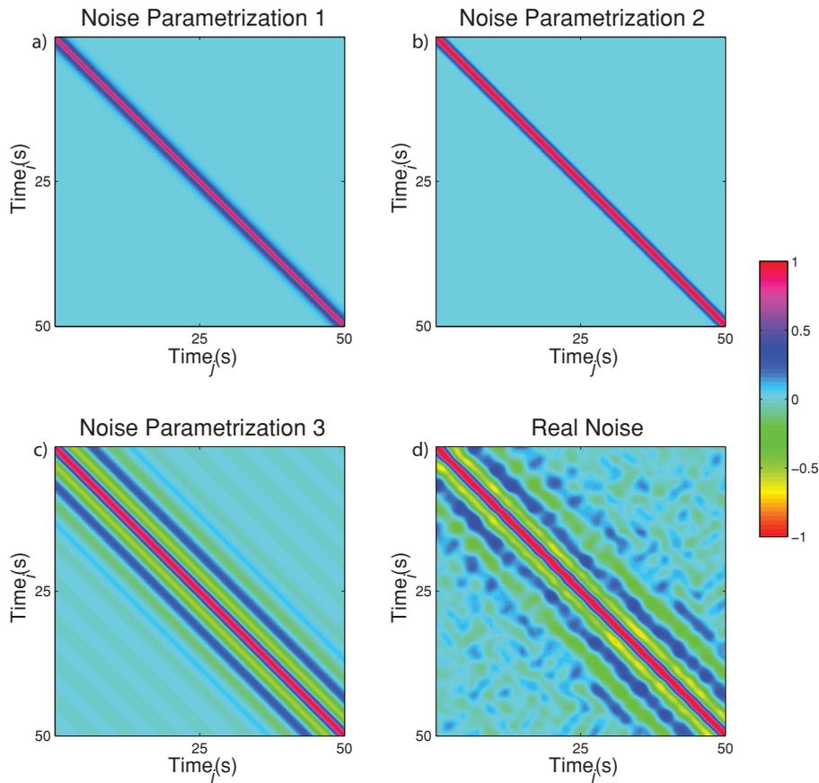
**Figure 4.** Covariance matrices from the three types of noise parametrization and actual noise. (a–c) Parametrizations 1–3. (d) Covariance matrix generated from pre-event noise at ANMO. The rate at which correlation decays with increasing lag times varies across the parametrizations; parametrization 3 (c) is most similar to the behaviour seen in real noise covariance (d), due to its ability to represent the microseism.
