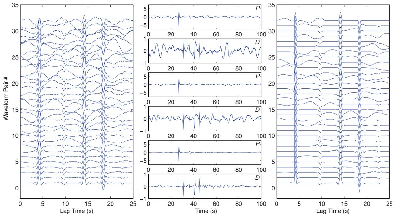
**Figure 8.**  $P_s$  waveforms and deconvolutions. Left-hand panel: the damped spectral division receiver functions for synthetic  $P_s$  seismograms with 32 increasing noise levels. Right-hand panel: the THBD receiver functions for the same seismograms. Central panels: the parent and daughter waveforms for waveform pairs 4, 17 and 30; note the increasing level of noise especially on the daughter component. The THBD method produces fewer artefacts than damped spectral division.
