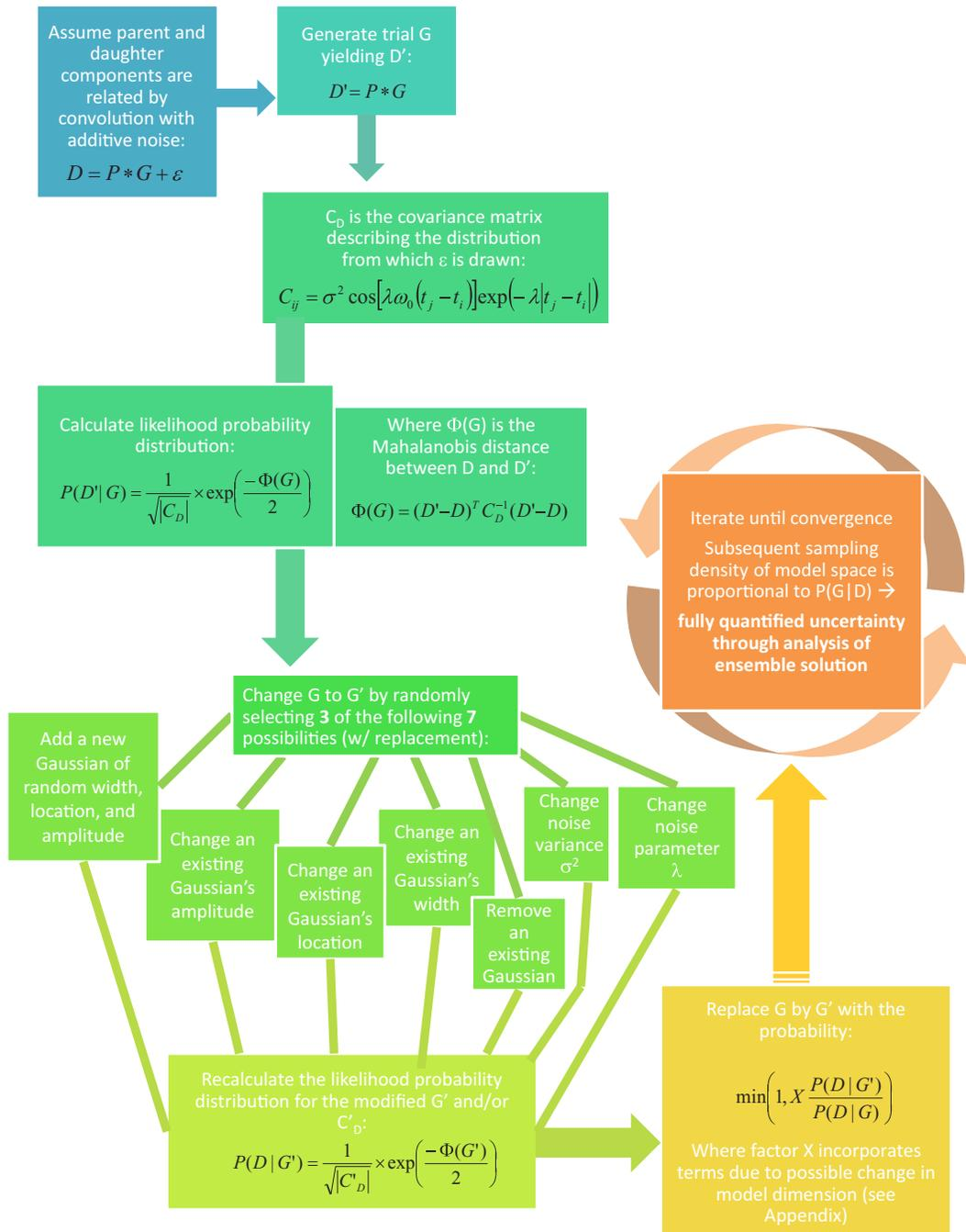
**Figure 1.** An overview of the reversible-jump Markov chain Monte Carlo algorithm used for our deconvolution. The  $C_{Dij}$  shown describes noise parametrization type 3. For parametrization types 1 and 2, see Section 3.
