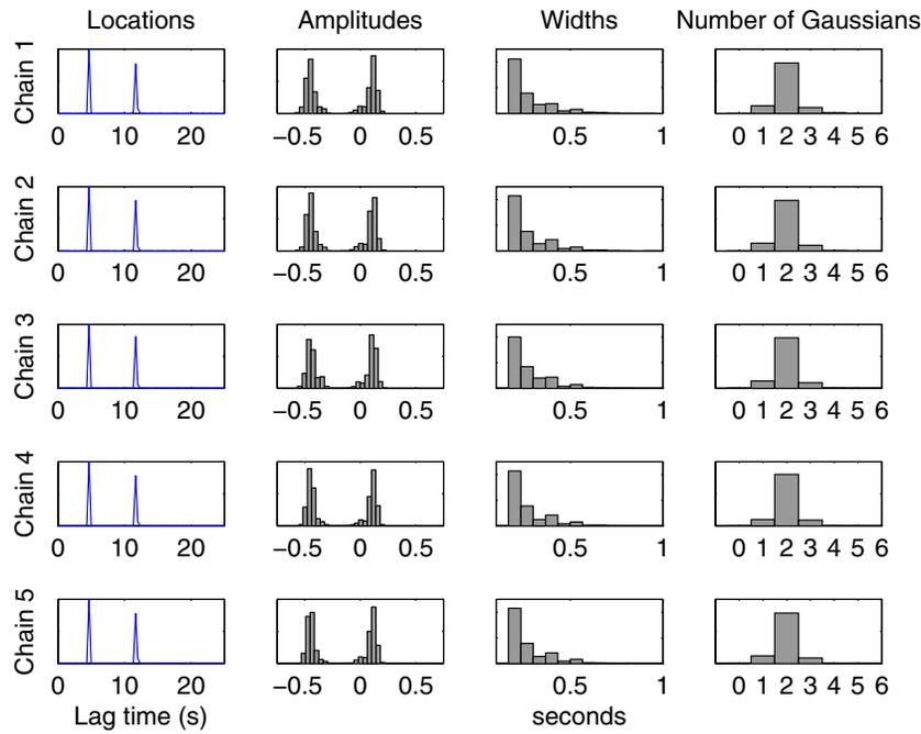
**Figure 3.** Histograms showing marginal densities of Gaussian locations, amplitudes, widths and number for five chains run in parallel on the same waveform pair. The fact that the parallel chains are sampling the same parameter values increases our confidence that the algorithm is successfully converging during the burn-in period.
