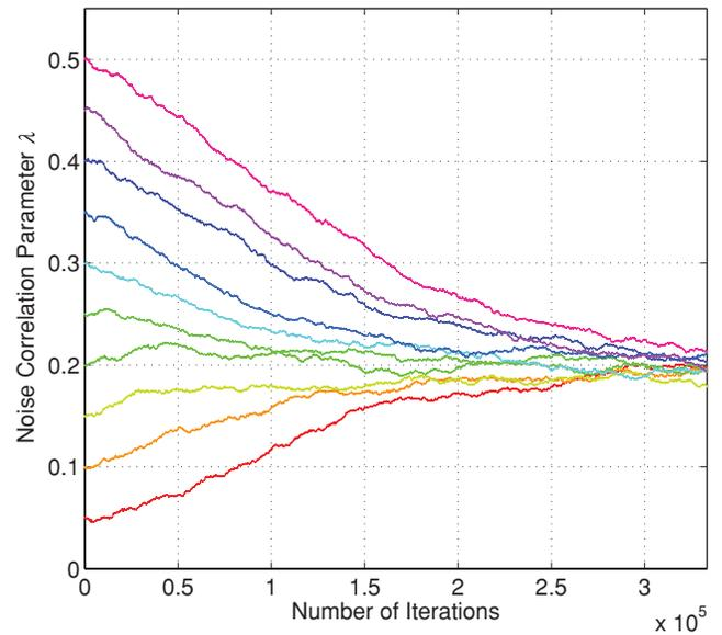
**Figure 14.** Noise correlation parameter  $\lambda$  by iteration. Markov chains with different starting values of  $\lambda$  are shown and all converge to  $\sim 0.2$ , the same  $\lambda$  value we found best fit the covariance matrix that was used to generate this noise. This illustrates that our method can successfully estimate the frequency content of the noise, parametrized by  $\lambda$ , even from inaccurate starting guesses.
