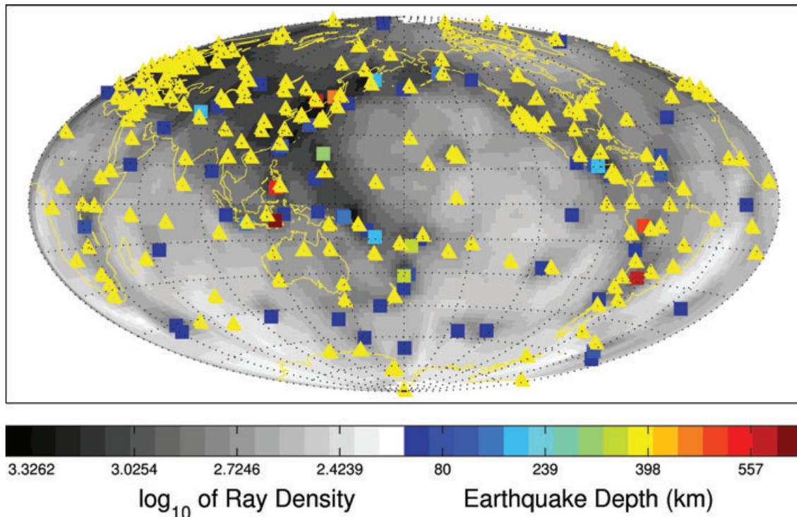
**Figure 6.** Map showing earthquake and station distribution of our synthetic data set. Earthquakes (squares) are colour-coded by depth, while the stations are denoted by yellow triangles. The shading is proportional to the log of the number of ray paths at that location.
