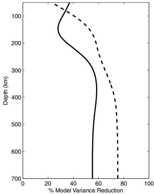
**Figure 10.** Relative variance reduction in percent resulting from the use of modified linear corrections for the  $V_s$  (solid line) and  $\xi$  (dashed line) structure as a function of depth.
