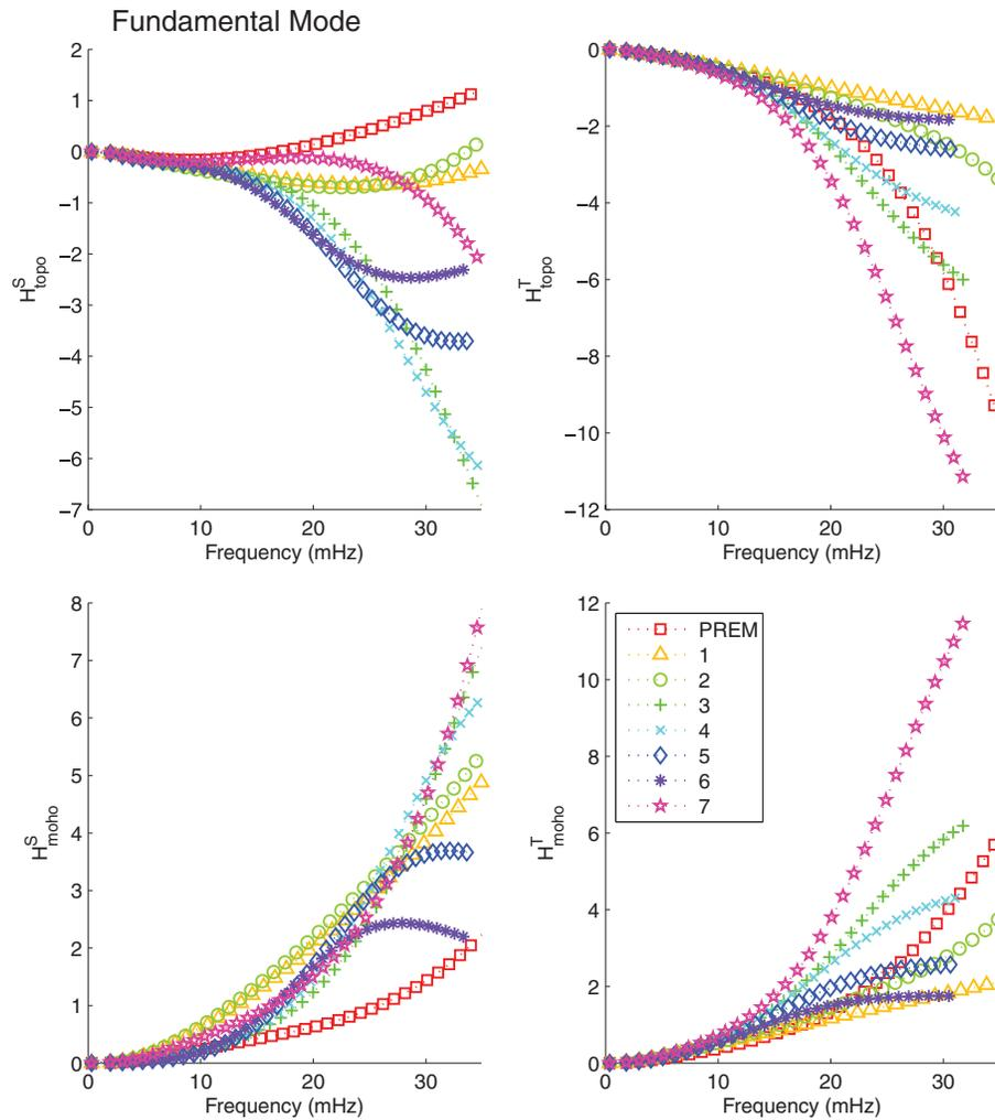
**Figure 2.** Discontinuity kernels  $H_k^d$  for surface topography (top row) and Moho depth (bottom row) as a function of frequency. Spheroidal fundamental modes are in the left-hand column, while toroidal fundamental modes appear on the right-hand column.
