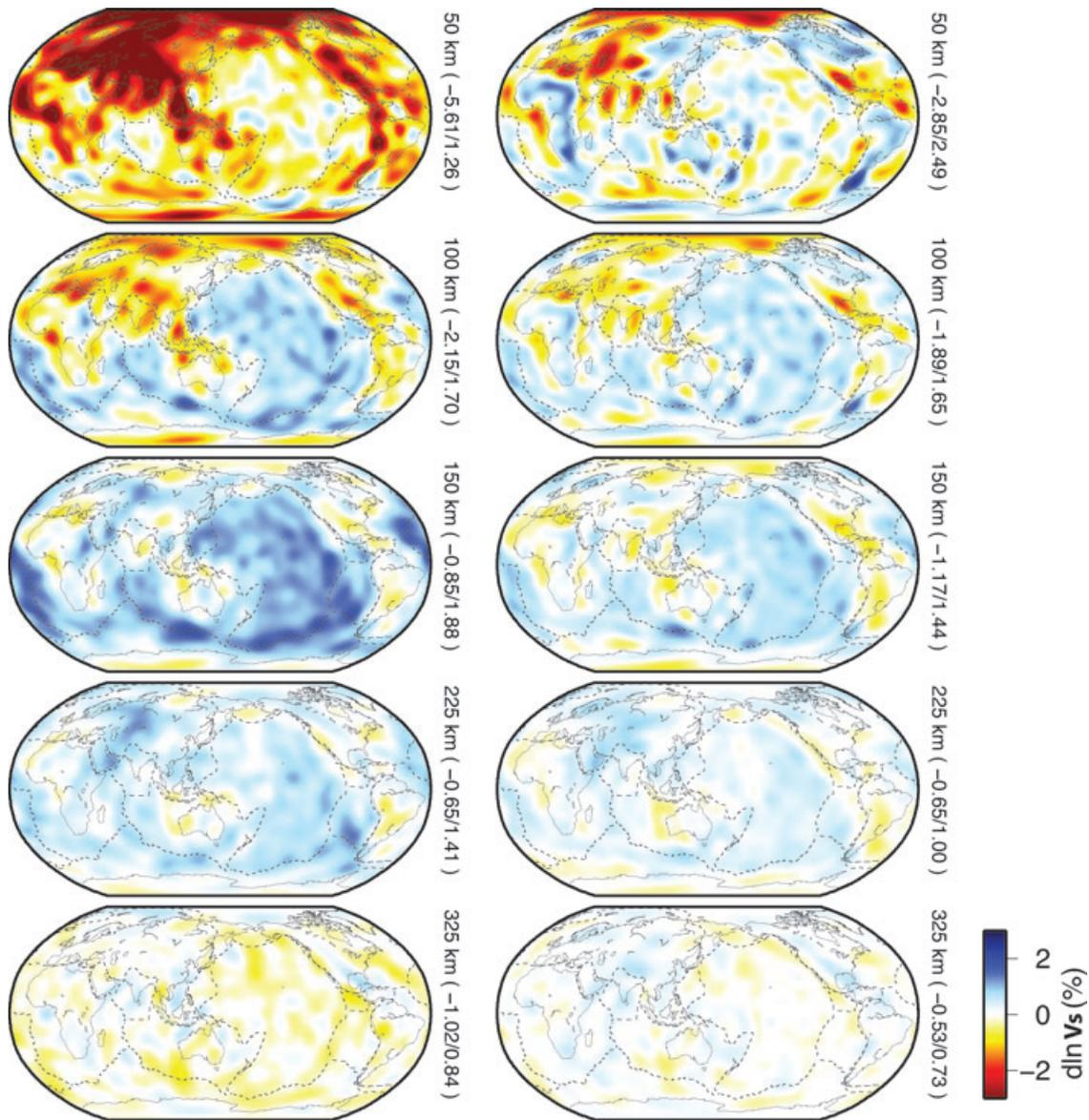
**Figure 8.** Expected contamination of mantle isotropic  $S$ -wave speed due to the use of standard (left-hand column) and our modified (right-hand column) linear crustal corrections on fundamental mode and overtone wavepackets. Warm (cool) colours indicate that using linear crustal corrections would artificially decrease (increase) retrieved mantle  $V_s$ . Note the significant amplitudes of contamination associated with standard linear corrections even at 150 km.
