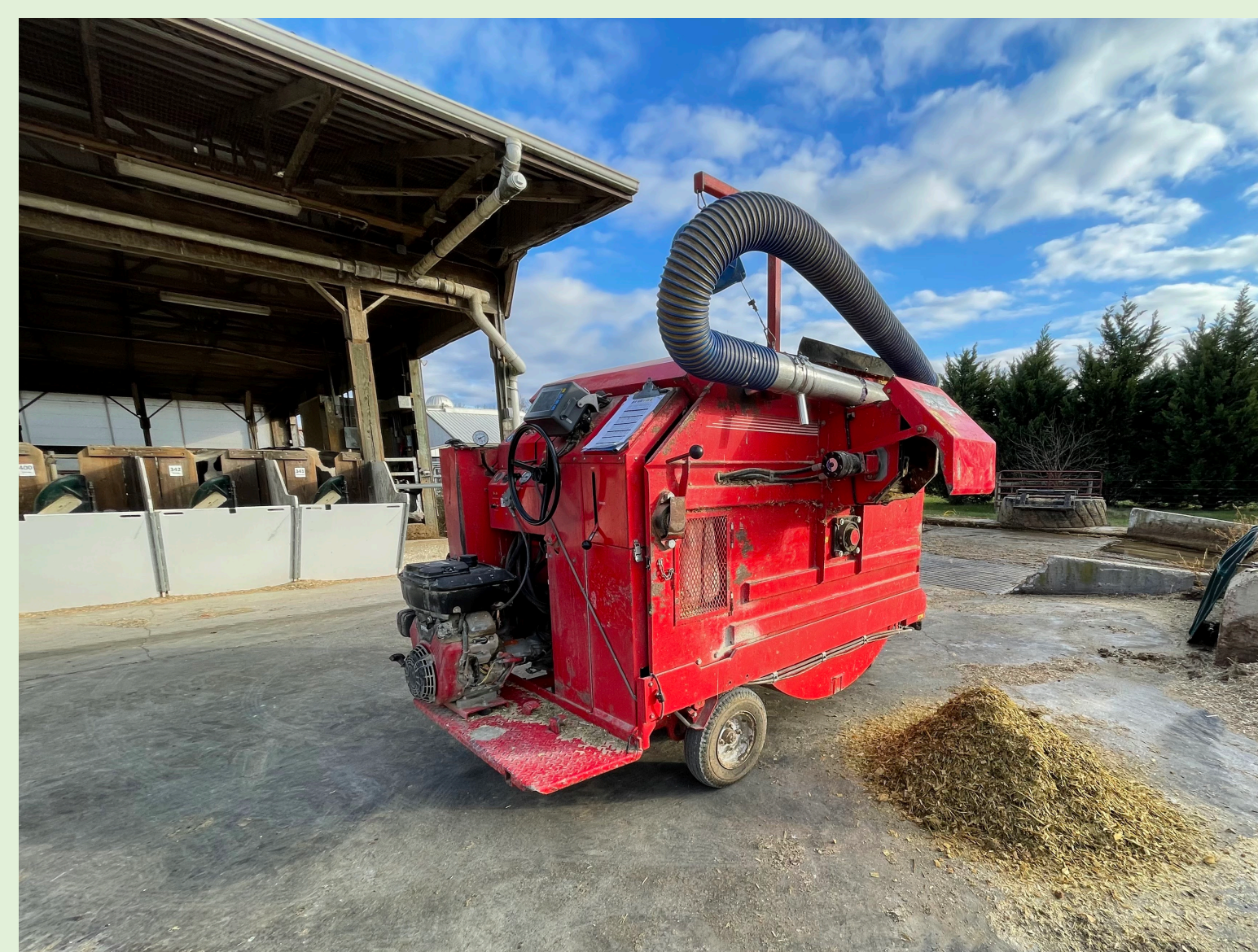
Image of the Calan data ranger used to collect, deliver, and record feed
