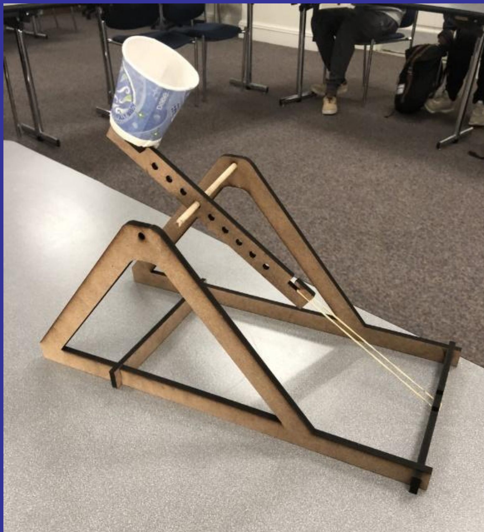
Here is a picture of our finished prototype for our catapult. It was designed with a lower cost in mind to be good activity in schools to introduce them to engineering.
