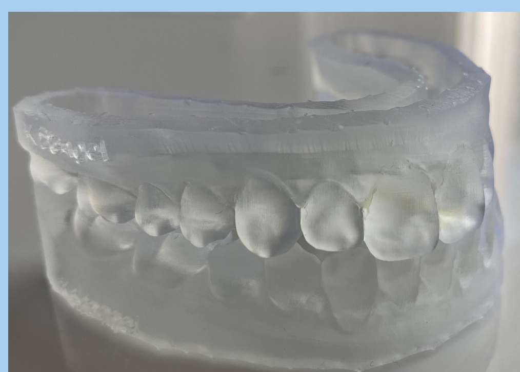
Image of a 3D printed tooth model used to make retainers for patients
