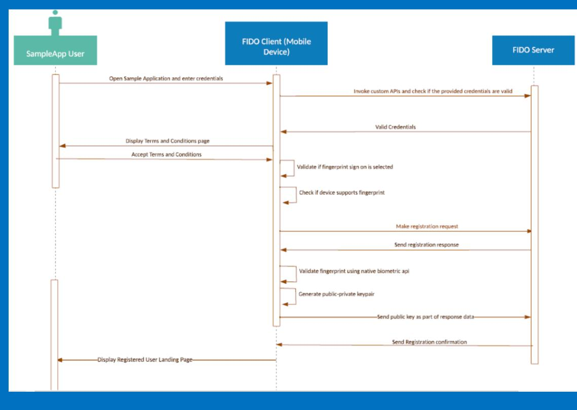
This is an example of the authentication workflow for a FIDO-compliant authenticator. It displays the interactions between the client, application, and server, that would take place during biometric (e.g. fingerprint) authentication. Image credit: PPS Infotech
