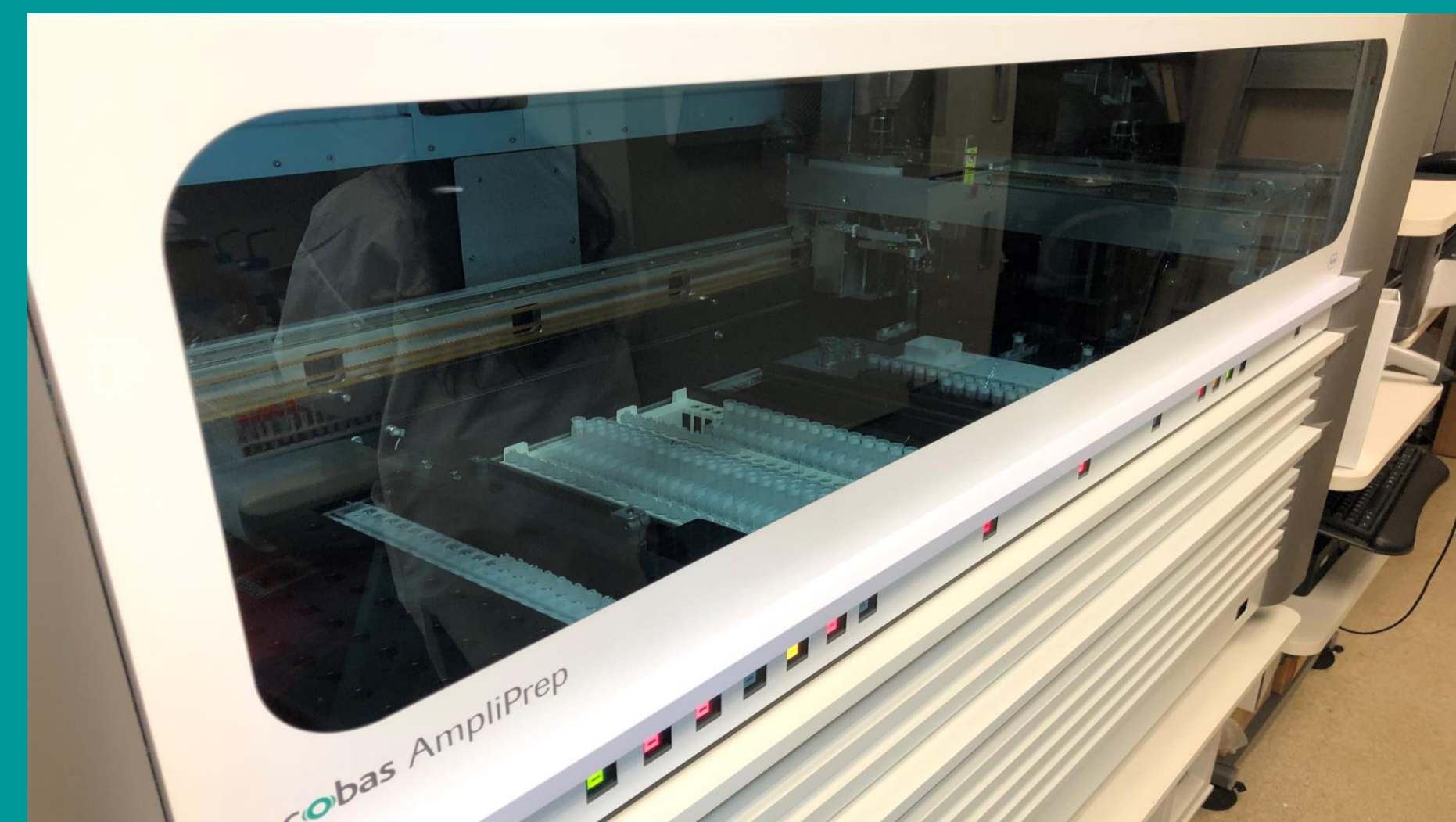
One of the many PCR machines in the lab. Polymerase Chain Reaction (PCR) is a method used to study DNA by amplify a small sample.
