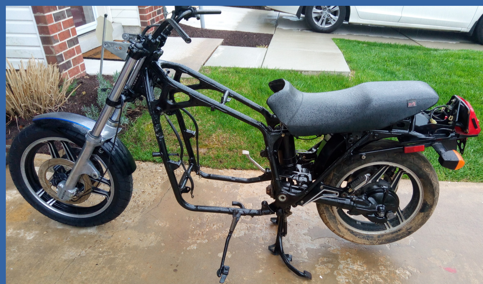
The new paint on the frame, polished forks, and the new front tire
