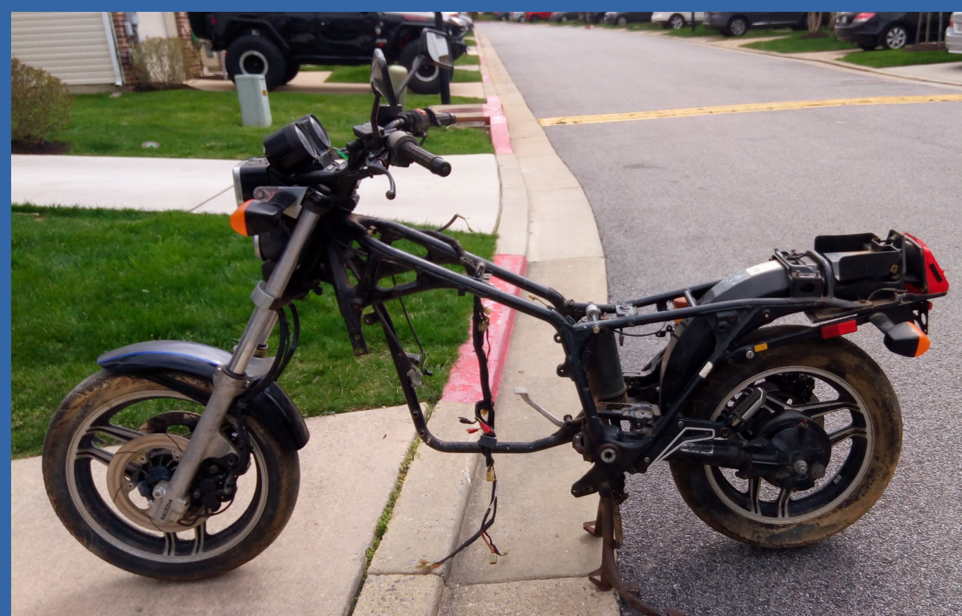
The engine and the left subframe off of the motorcycle
