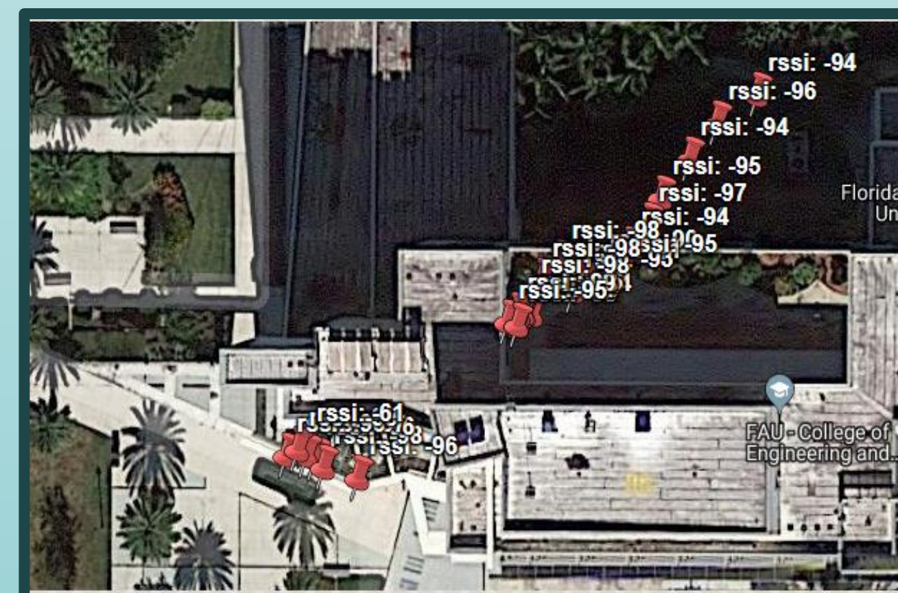
Area where signal was received from node. Each pinpoint shows measured signal strength from GPA coordinate
