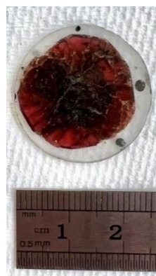
Figure 5: A portion of sample preparation. Garnets from Garnet Ledge were measured, photographed, and then mounted in dental resin.
