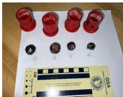
Figure 5: A portion of sample preparation. Garnets from Garnet Ledge were measured, photographed, and then mounted in dental resin.
