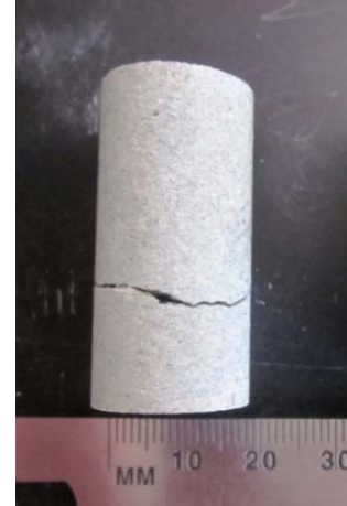
Figure 3: Soapstone sample fractured with a low confining pressure of 300 kPa.
