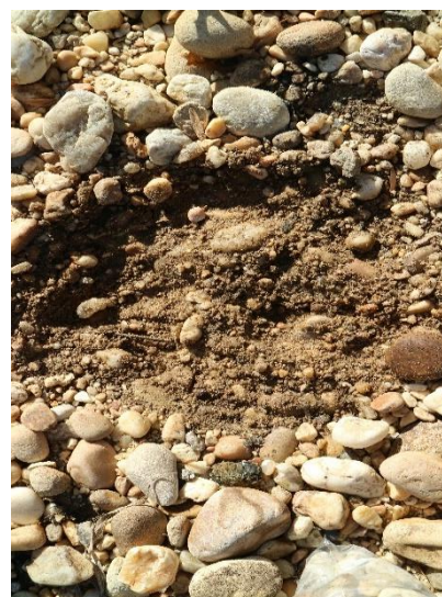
Figure 9: Exposure of subsurface sediment where the surface has been scraped away for grain size analysis, note the significantly lower quantities of large cobbles and higher quantities of sand and silt in the subsurface. Photo By: Patrick Deery
