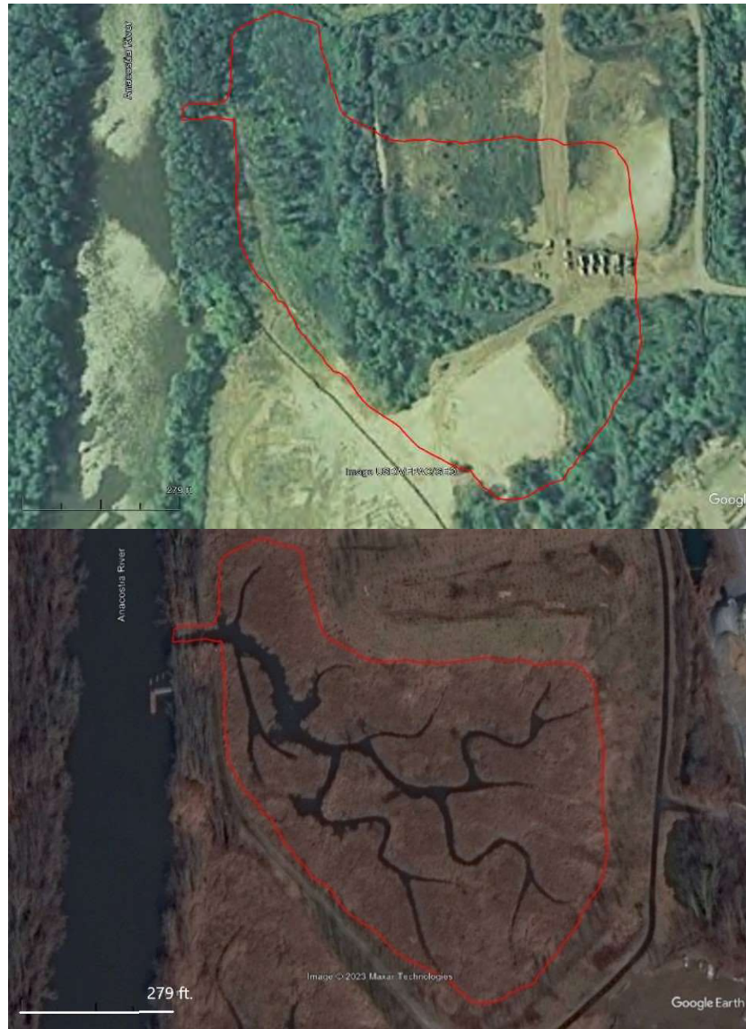
Figure 2: Top: Google Earth air photo from 12/2008 of the marsh location before construction. The red outline has an area of 39,000 m 2 and depicts the future location of the marsh. Bottom: Air photo from 1/2017 of the constructed marsh with the same red outline from the image on the top.
