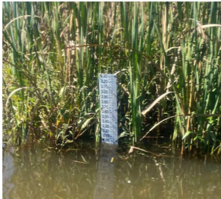
Figure 5: Tidal stage measurement using a USGS staff gage.
