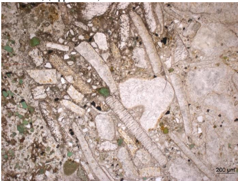
Figure 10: Thin section from the Chuskuna Formation (plane polarized light). Glauconite is the green mineral, seen primarily on the left side of the image.
