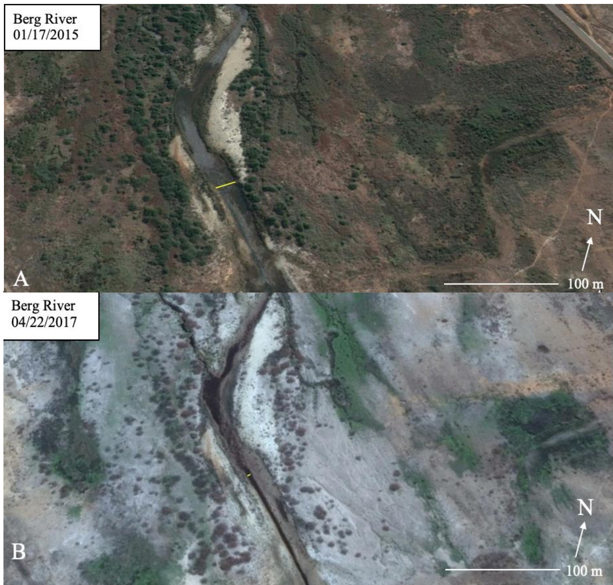
Figure 16 Site along Berg River where wetted width measurements were taken in (A) Wet Year and (B) Dry Year. Yellow lines represent wetted width. The site is approximately 0.65 km downstream the Berg River Dam.
