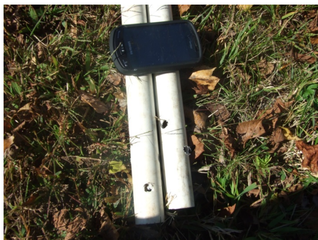
Figure 6: the PVC pipe posts created, with holes drilled into the top, allowing strings to be tied
