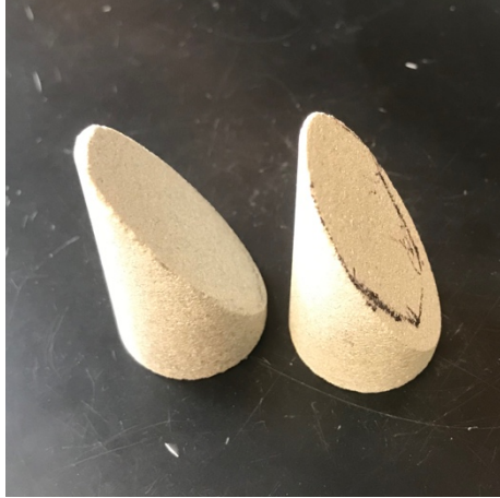
Fig 5: Berea Sandstone cylinder cut into two equal parts at 30° angle. Cylinder is put back together after gouge layer applied.
