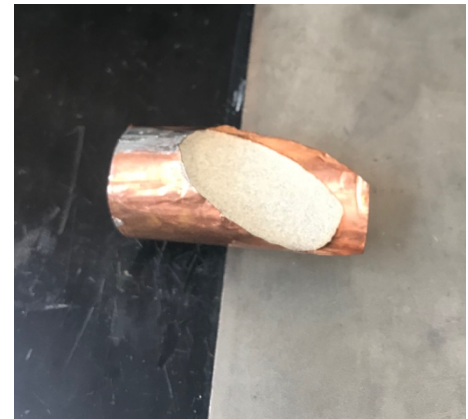
Fig 6: One half of the Berea Sandstone wrapped in the copper foil. The gouge layer was applied and allowed to dry before being sealed with the other half.
