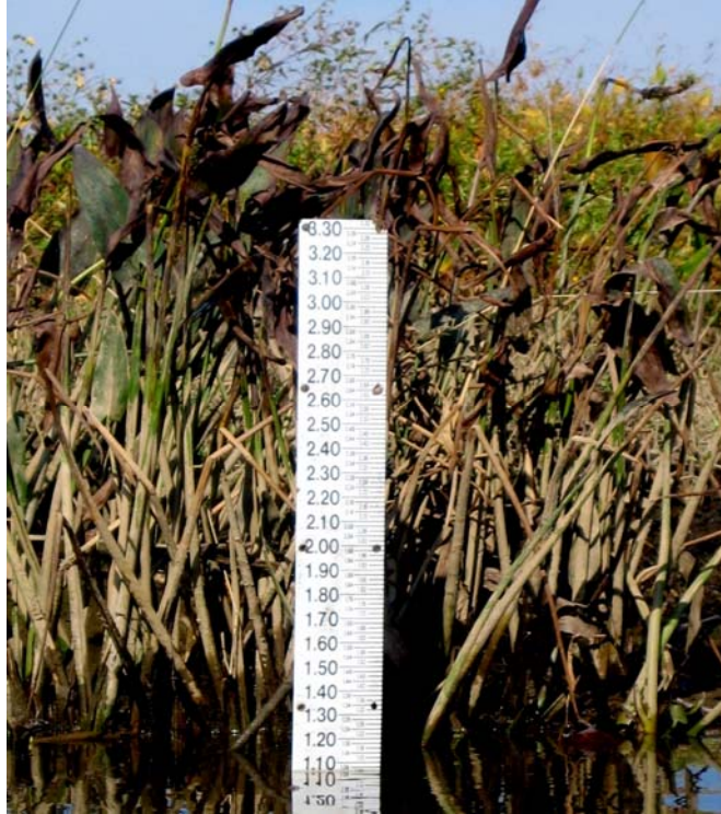
Figure 6: Tidal stage is measured with a staff gauge
