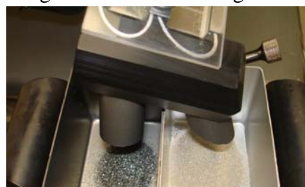
Fig. 4. magnetic grains left, non magnetic right.
