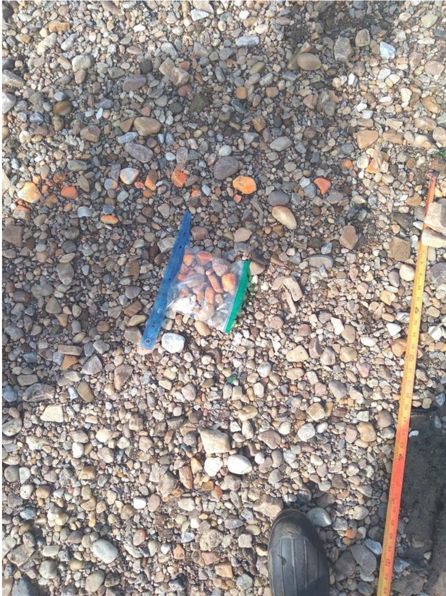
Figure 7: Particle Tracers. Orange pebbles are the tracers.
