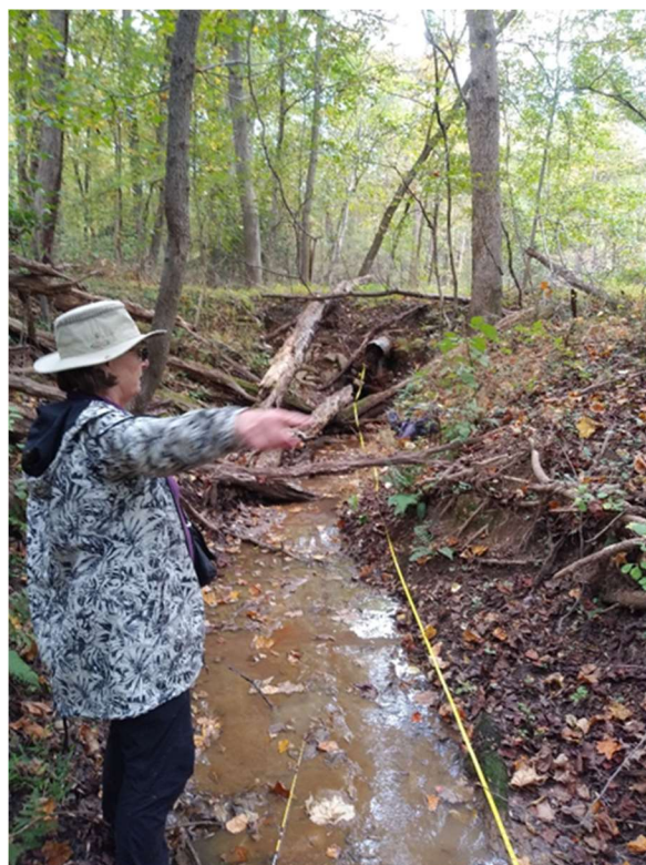
Figure 9: Laying the tap measure parallel to the incised stream's bankfull flow path as part of a longitudinal profile survey (Dr. Karen L. Prestegaard for scale).
