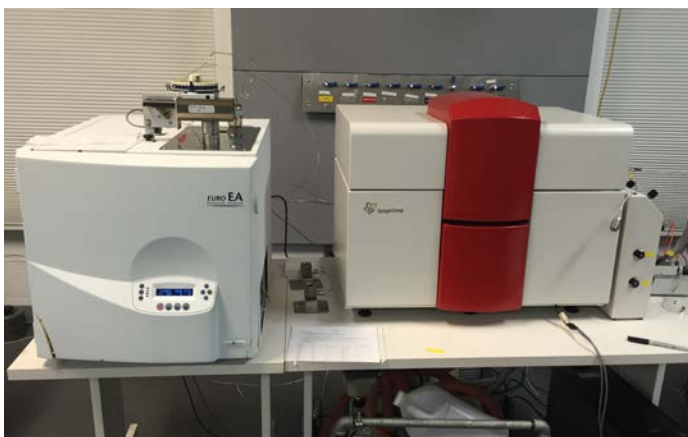
Figure 8: The Elemental Analyzer (left) and the Isoprime Mass Spectrometer (right).
