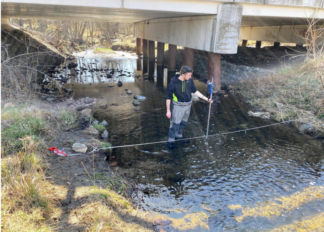
Photograph 5. Stream velocity measurements taken with an acoustic velocity flow meter at Site SLB5. Photograph provided by Christiana Hoff. Additional photographs of measuring stream velocity available for reference in Appendix B.
