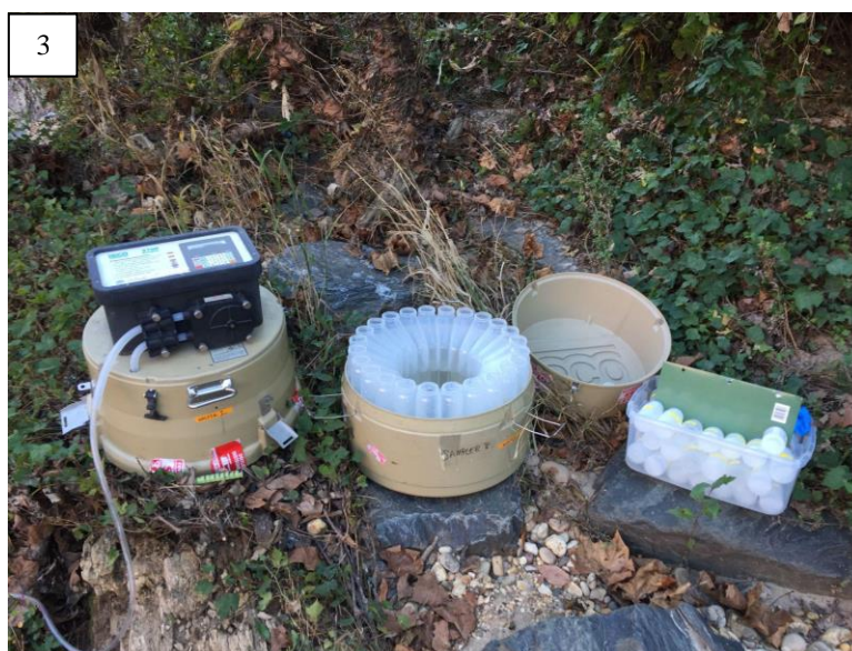
Photographs 2 and 3. Photographs of automated samplers in the field at Sites SLB10 (Left) and PB8 (Right).
