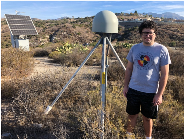
Figure 7: A photo of the WHYT GPS station in Southern California with myself as a scale. USGS has thousands of GPS stations spread across the state just like this one. The half-domed structure at the top is the GPS receiver, while the angled posts are meant for support. The station has a central pylon drilled into the bedrock for stability and to prevent inaccurate readings from erosion, wind, or human or animal activity which could otherwise rattle the station. Note the solar panel and radio transmitter in the background (left). The radio transmitter sends data via satellite to the USGS office in Menlo Park, California for processing.
