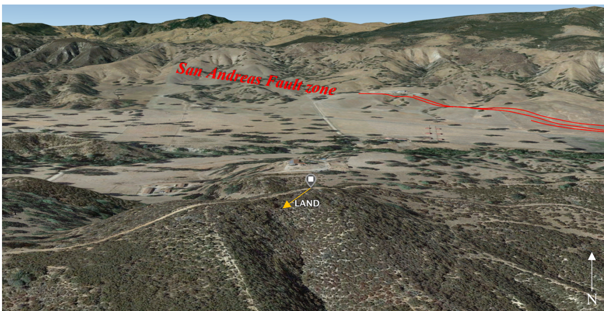
Figure 12: Google Earth image of the LAND station on top of a small peak, overlooking the San Andreas Fault zone (in red). The orange vector is representing the direction in which the LAND station calculated orthogonal motion with respect to the San Andreas Fault in the month timeseries. The steep terrain in the foreground caused some creep rate measurements to be difficult to determine due to minor landslides in part because of the moderate shaking from the 2019 Ridgecrest earthquake sequence.
