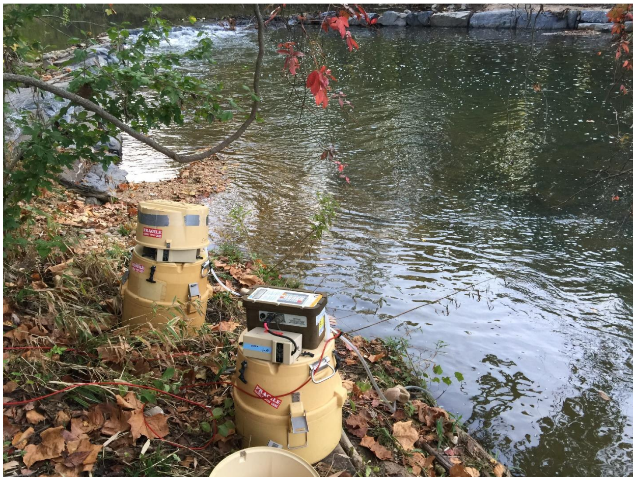
Figure 3. Automated sampler ISCOs are set up along the bank of the Northeast Branch Anacostia River at Riverdale, MD. Each ISCO can hold up to 24 samples and two are therefore needed to take a 24 hour sampling period at 30 minute intervals. Each water sample had a volume of 250 mL. To minimize tampering, the ISCOs were located away from the nearby path and locked to a tree.
