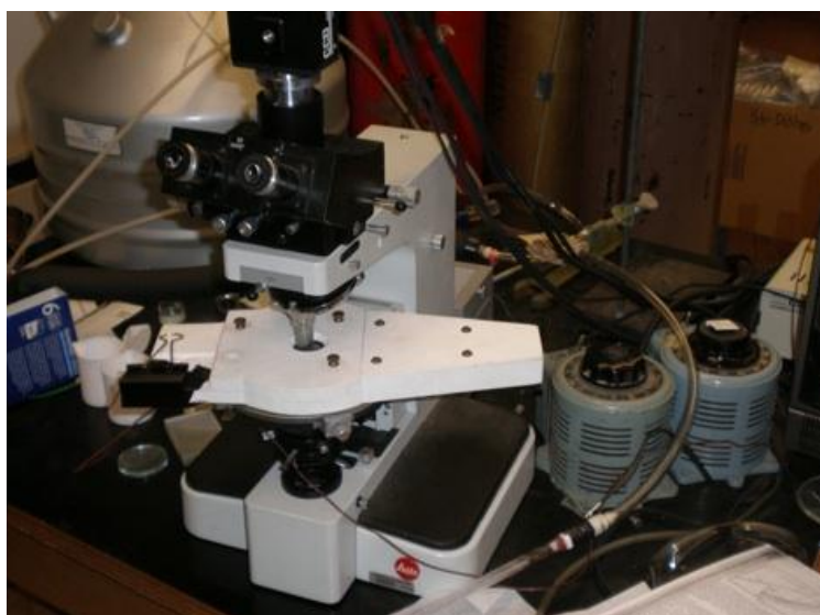
Figure 4: USGS-type gas-flow fluid inclusion stage attached to an optical microscope in the Laboratory for Mineral Deposits Research at University of Maryland. Photo by Dr. Brian Tattitch.
