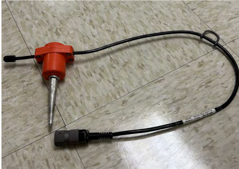
Figure 5. Example of a geophone used in the active source experiments.
