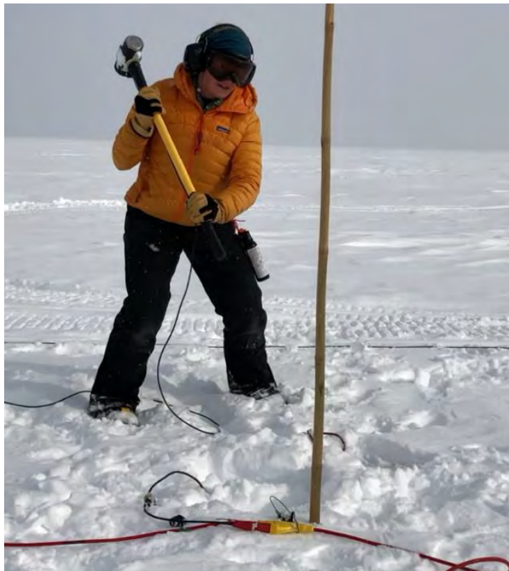
Figure 6. A member of Dr. Schmerr's team (Dr. Erin Pettit) conducting the hammer strike of the active source experiment.
