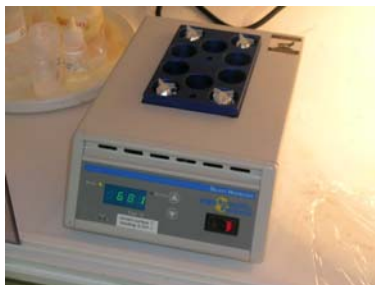
Figure 14. Inverted conical vessels wrapped in aluminum foil and heated in a heat block during Osmium Micro-Distillation.
