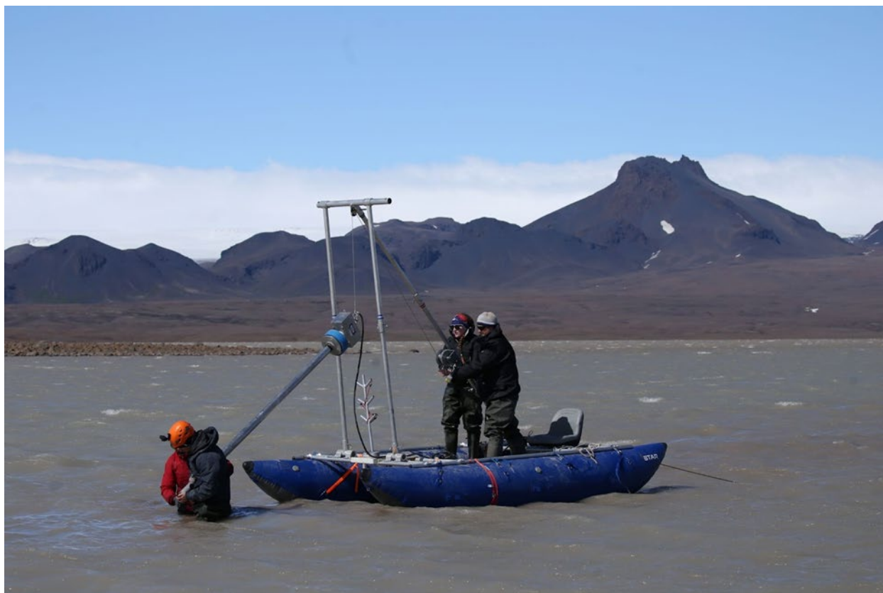
Figure S2: The floating drill rig used by the DIGMARS team to collect samples at Lake Sandvatn.
