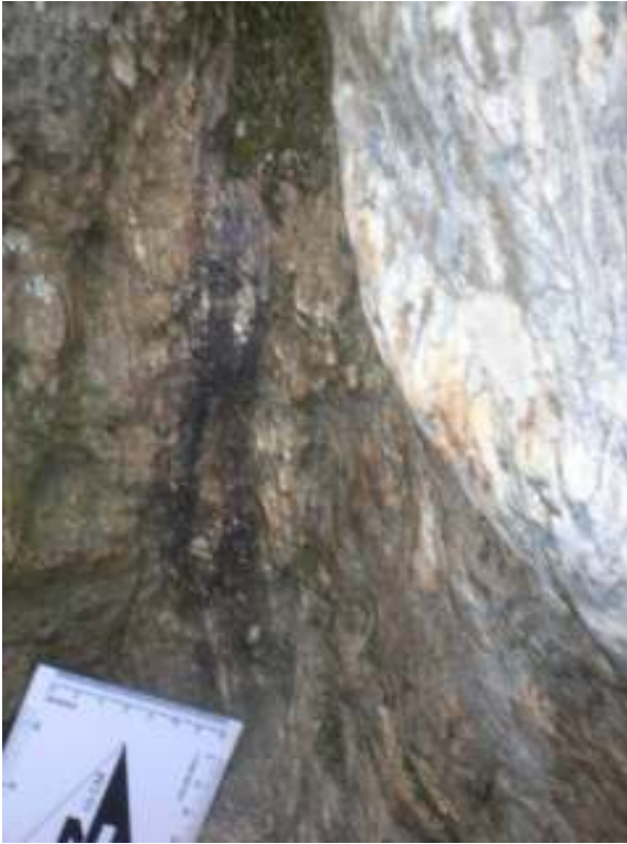
Figure 19. This is a close up photograph of a possible fault breccia found in a continuous fracture on the Rocky Island. The arrow is pointing to the dark region that may be breccia. The photograph was taken facing upstream.
