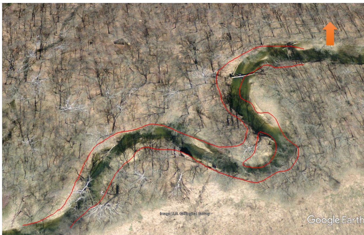
Fig. 7: Channel Boundaries from the 4/2008 channel shown on the 4/2018 image (drawn in Google Earth, the image is from the USGS for both years, the orange arrow is north direction). Note the cut-off chute that was formed and subsequently reconnected in the middle of the bank.
