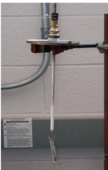
Figure 4. A demonstration of how the silica tubes were hung with platinum wire in the hot spot of the furnace.
