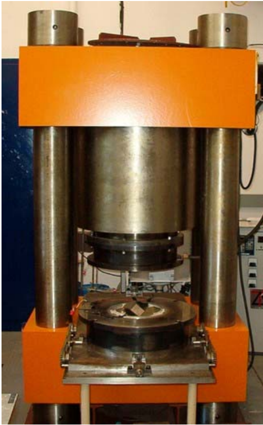
Figure 7. The multi-anvil apparatus used for the 6 GPa experiments.
