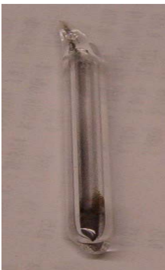
Figure 3. A sealed silica tube with sample powder. This tube was hung in a Deltech vertical furnace until equilibrium was established.
