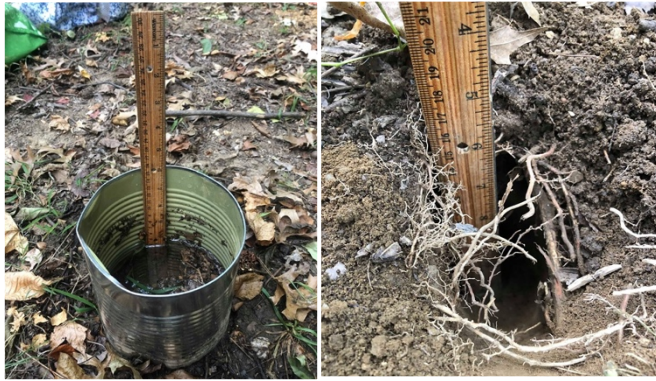
Fig. 8: (Top) A 15.5 cm single-ring infiltrator during an infiltration test. (Bottom) Measuring the wetting depth, and numerous roots just under the ground surface.
