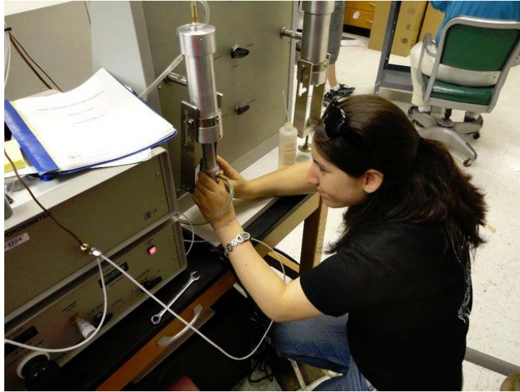
Fig. F: Operation of the permeameter. The aluminum rod I am holding pushes the rock core into the vacuum chamber above. Pressure is set in the chamber and helium gas is shot upstream, measuring the flow rate (and subsequently, permeability) of a rock.
