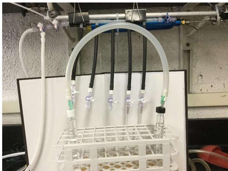
Image 1: Experiment set up. Black tube flushes nitrogen into left tube (tubes one-four in experiment) and sulfur dioxide gas is purged into tube on right (tubes one 'a'-four 'a') which is oxidized and precipitated as barite.
