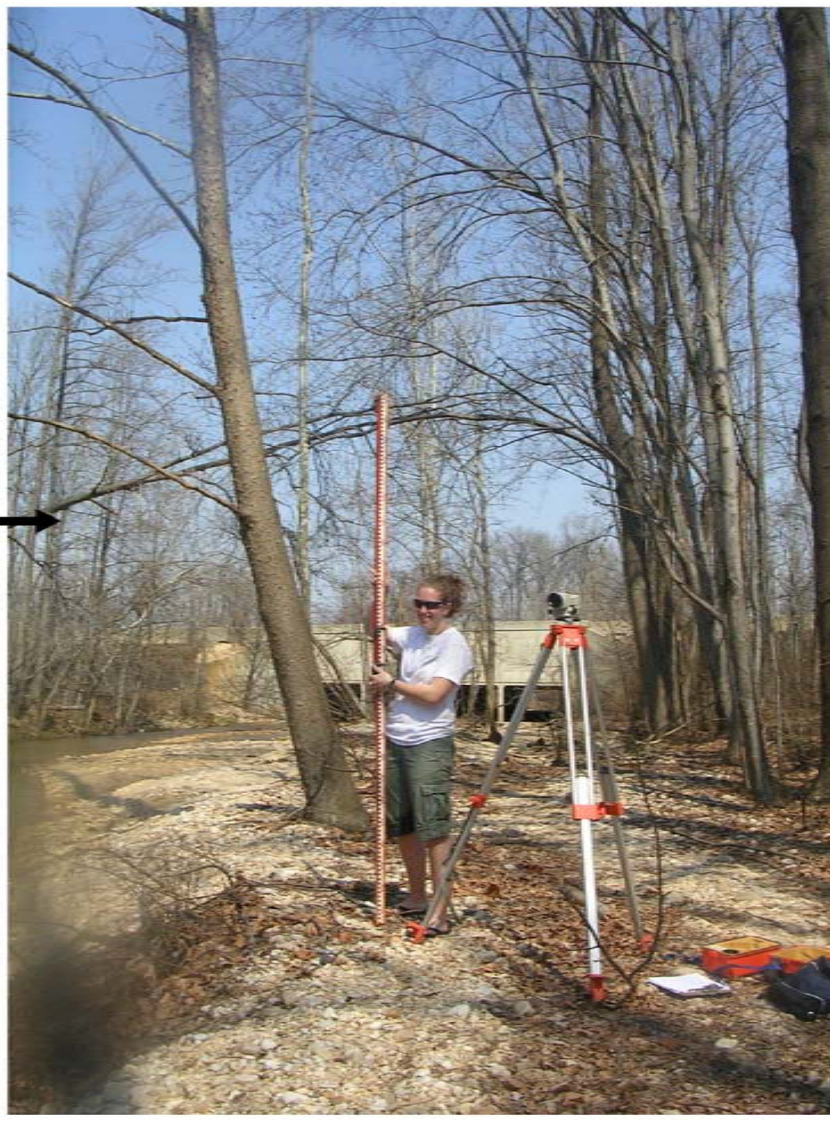
Field equipment: Stadia rod (2 meter) and surveyor's level
