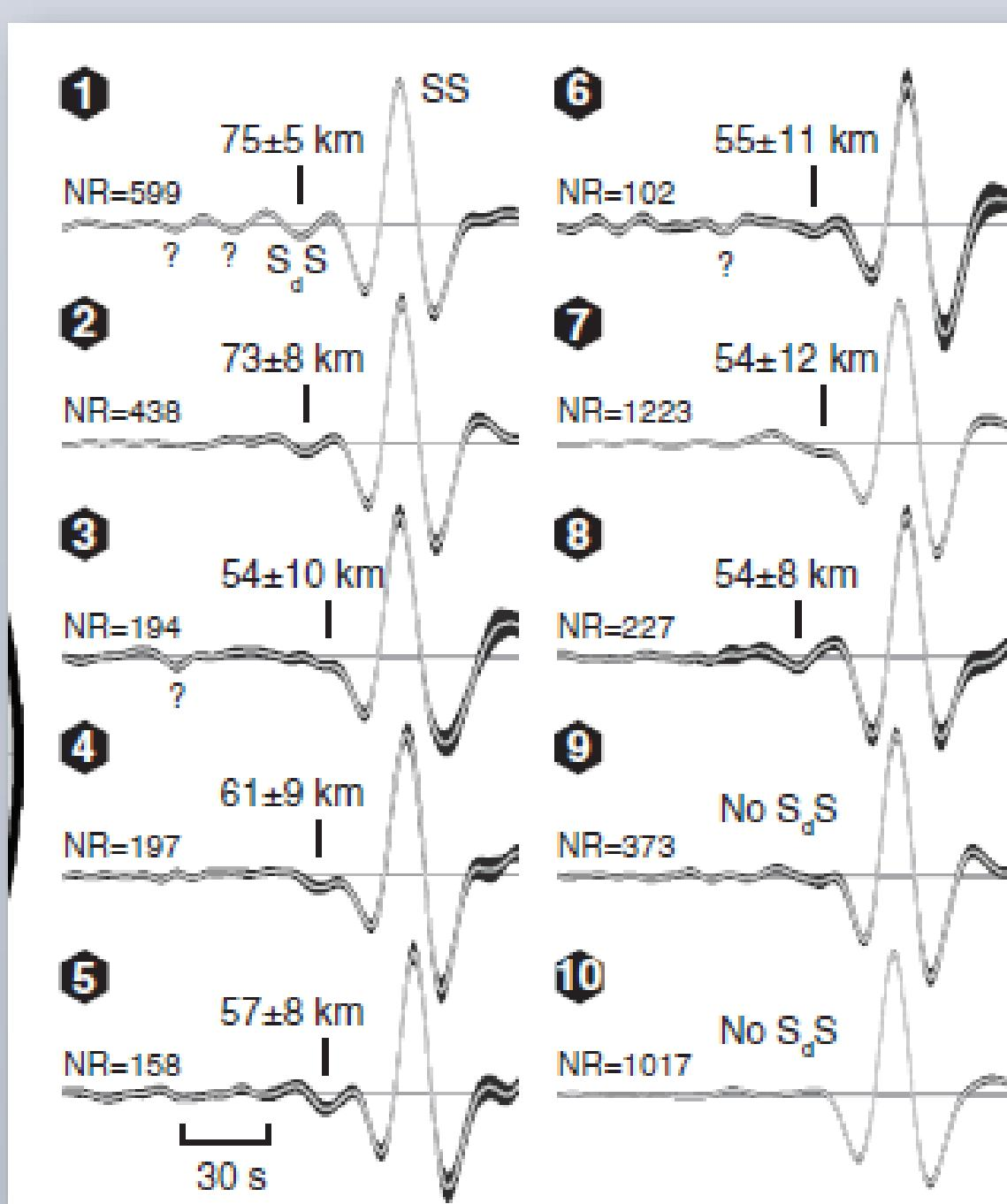
The figure to the left shows example stacks from detecting G in the Pacific. The maximum amplitude of each stack is normalized to unity. Amplitudes are displayed relative to the zero line. Shading shows statistical variation in combined stacks, anything that falls within the gray is 2 sigma with 95% confidence, and if it does not, it will be considered background noise.
