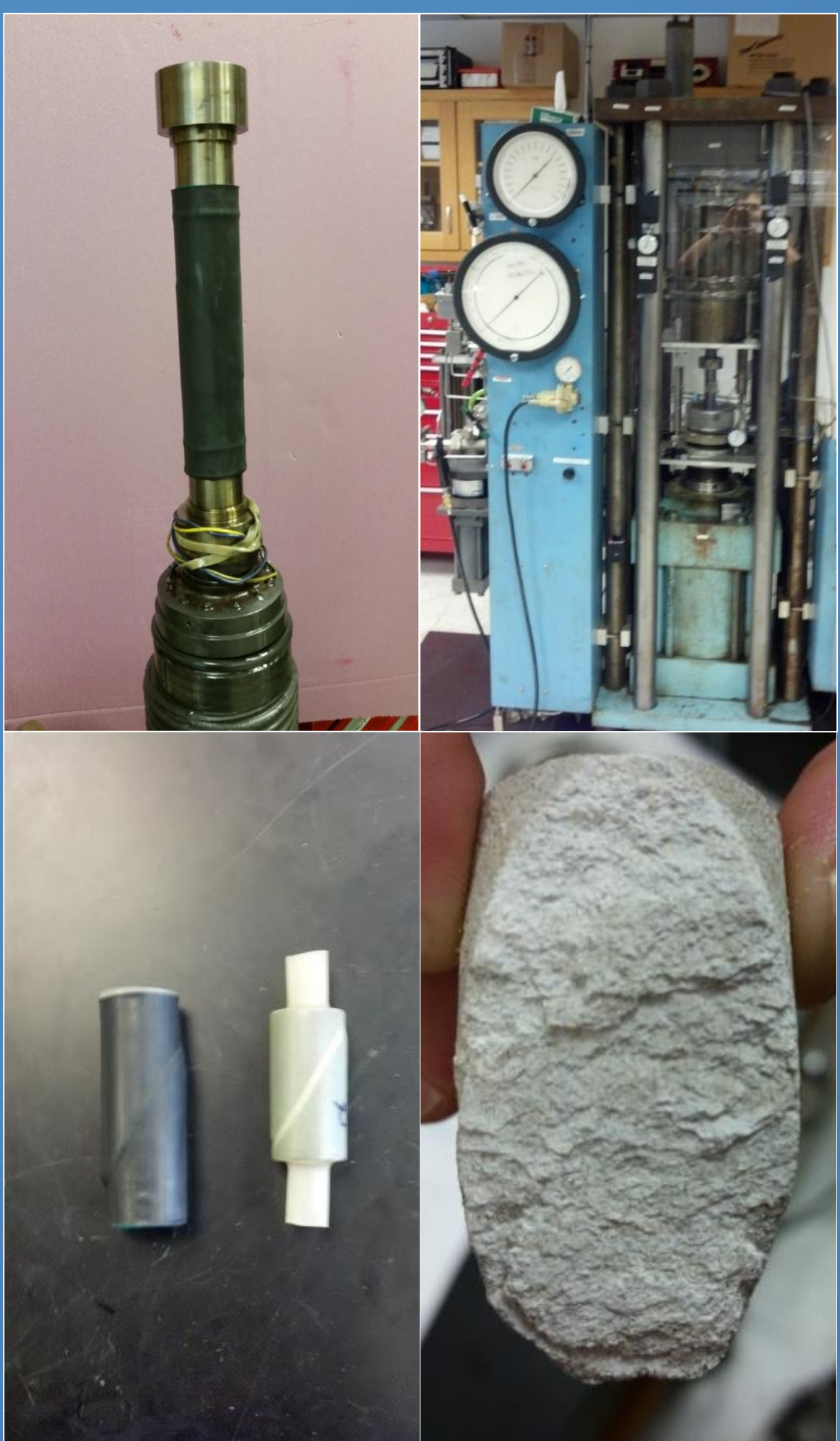
Upper Left: Sample that is almost finished preparation. Upper Right: Tri-axial Deformation machine. Lower Left: Sample after deformation. Lower Right: Face of a sample after deformation.
