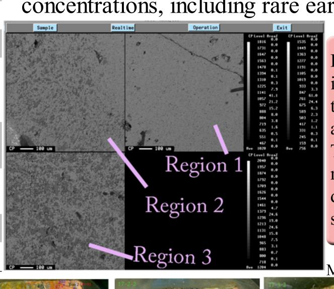
Backscatter electron (BSE) image of 16-4-1. Albitization (darker phase) is variable across a single sample. This albitization is macroscopically visible as dark and light epidotes in sample 16-4-1 below.
