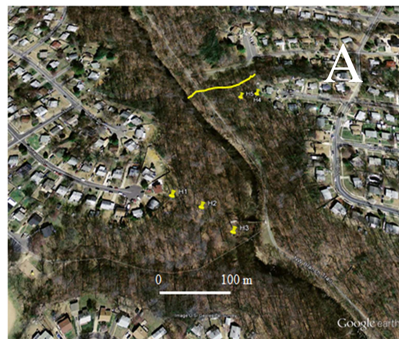
Fig. 2A: Yellow line shows the path of the 1 st order channel in the location of the Adelphi subdivision (~ 1950's) near the NW Branch of the Anacostia River. The yellow pins indicate the locations the samples were collected. The red arrow shows the direction downstream. This channel was made in the 1950's.
