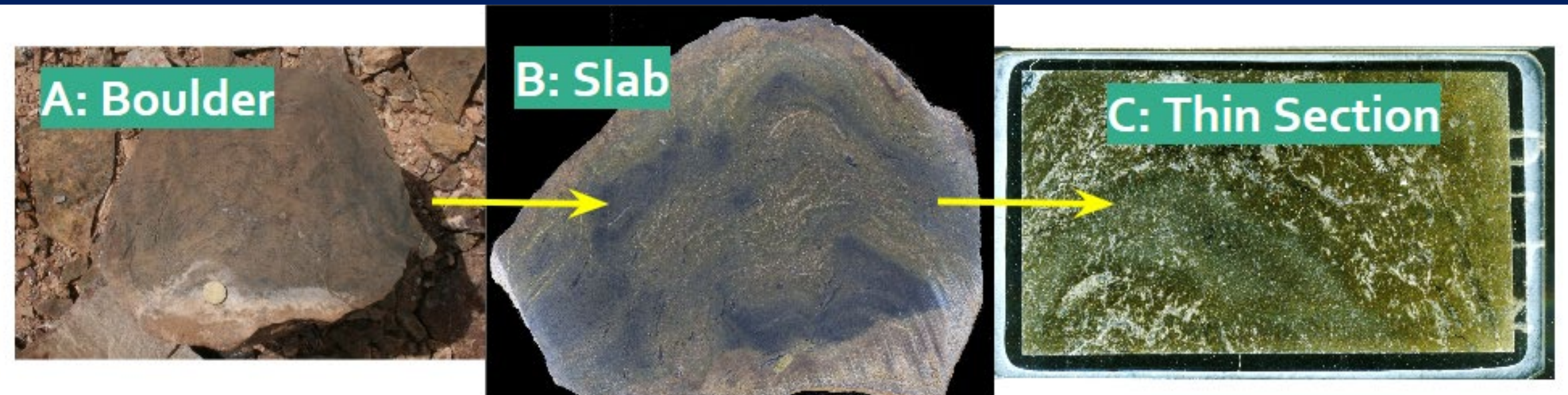
Figure 1: Samples. 1A: Boulders were analyzed at the micro- and macroscopic levels. 1B: Cross sections of boulders (slabs) were analyzed with a micro-XRF spectrometer at the cm-scale. Slabs were also micro-drilled for \delta^{13}\text{C} and \delta^{18}\text{O} analyses. 1C: 30- \mu\text{m} thin sections were analyzed with a petrographic microscope and an EPMA at the mm-scale.
