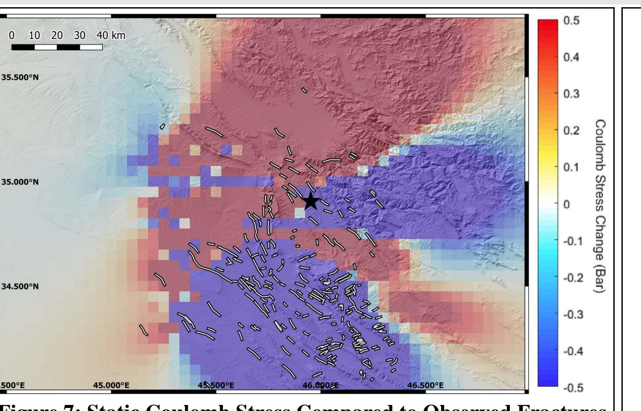
Figure 7: Static Coulomb Stress Compared to Observed Fractures
