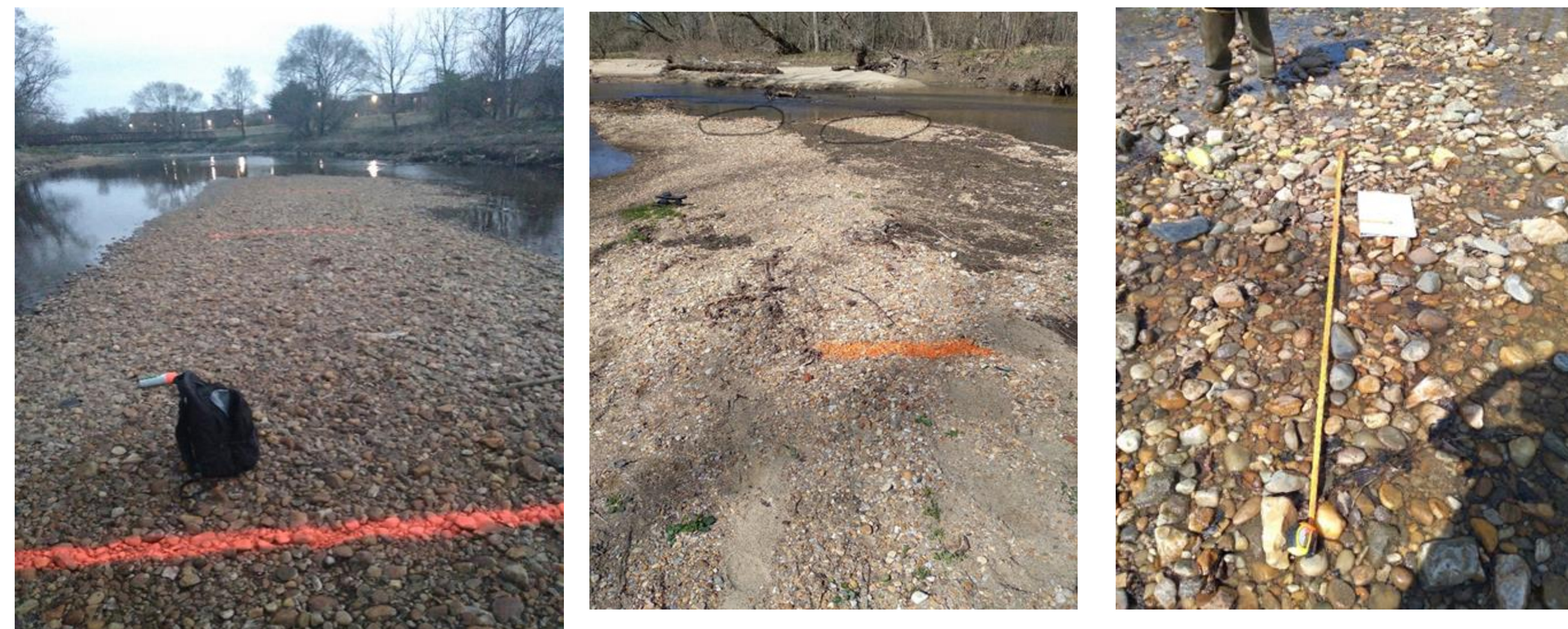
Fig. 3: Left: Marked Particles in channelized reach (3 per bar on 2 bars); Middle shows alluvial reach, Right: Alluvial reach measurement of the distance each particle traveled (Right)
