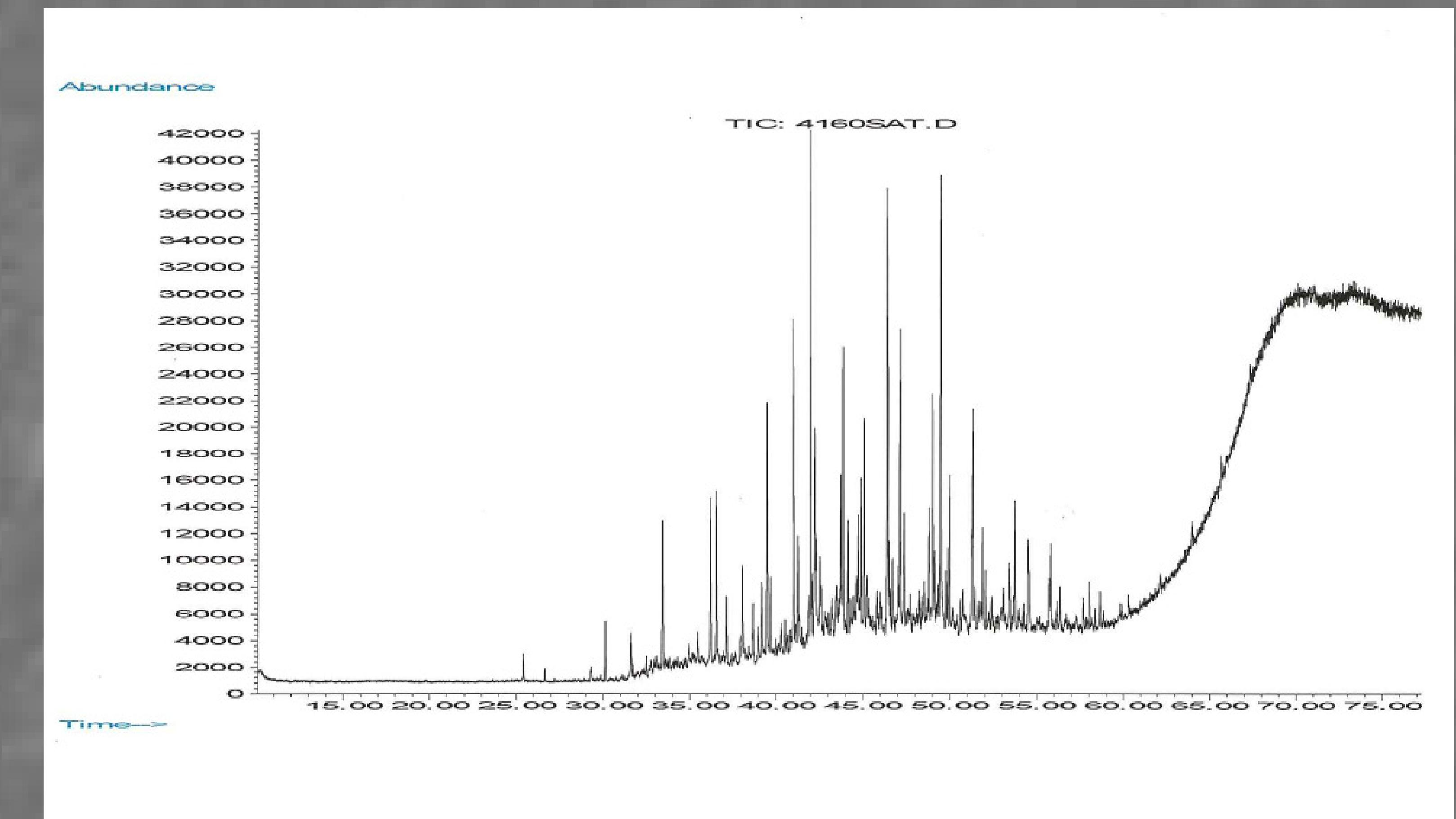
This is the original chromatogram for sample 41.60. 41.60 is the depth of the sample in meters. SAT is written at the end of the sample to denote the sample being run through the GC-MS is the saturated fraction. During this run, there was an issue with the GC-MS and pieces of the column falling into the sample and being counted as data.
