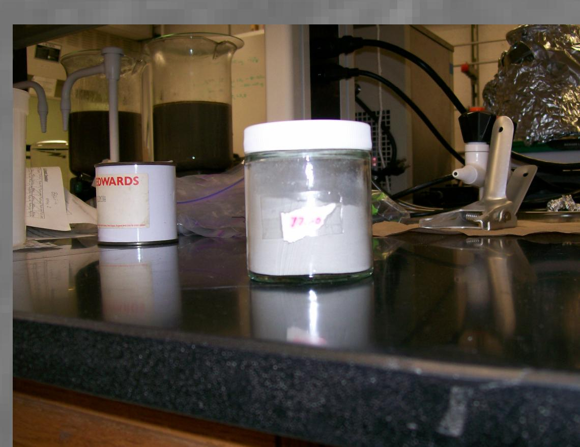
Approximately 100g of each sample were taken from the core. The outer 0.5 cm was removed first, and then the sample was broken in 0.5 cm<sup>3</sup> pieces. These pieces were cleaned with Milli-Q water and dipped in dichloromethane. The cleaned pieces were then crushed into powder using a mill and puck shatter box. All of my samples have been crushed by Kristen Miller. Next the samples will be extracted.
